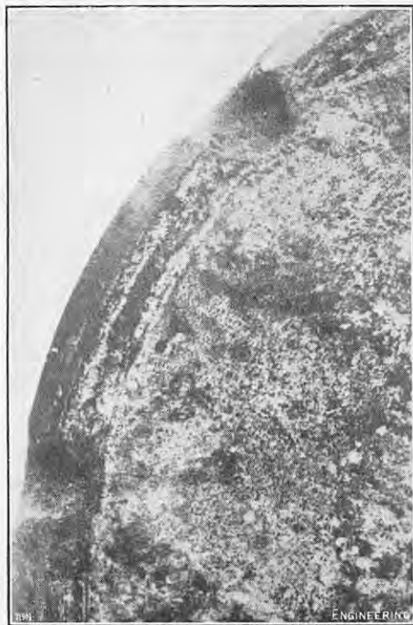
FIG. 8. GUTTERS IN EXHAUST-VALVE FACE.
