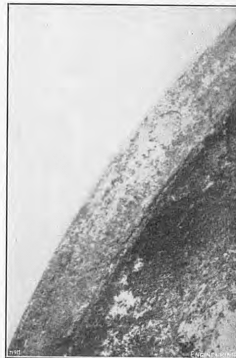
FIG. 7. DEPOSITS ON VALVE FACE.
