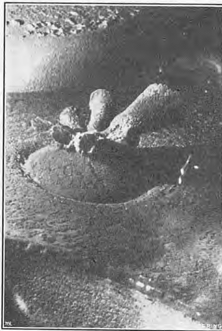
FIG. 6. INJECTOR TIP DEPOSITS AFTER SIX HOURS ON HEAVY FUEL.
