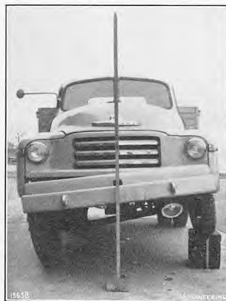
FIG. 2. SHOWING CHASSIS-FRAME MOVEMENT RELATIVE TO CAB.
