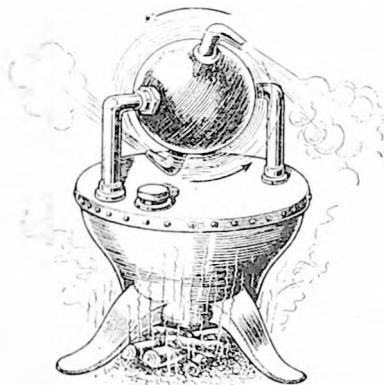
A model of the reaction turbine built by Hero, of Alexandria, in A.D. 50. Present-day turbines are developments of Hero's invention, but very different in appearance and efficiency.
