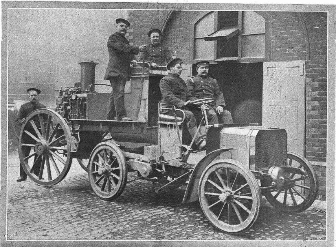
A MOTOR TRACTOR FOR FIRE ENGINES. This machine has been built by the Wolseley Tool and Motor Car Co., for the London County Council Fire Brigade and has been officially delivered to the Brigade at the headquarters in Southwark Bridge Road. The engine is a 24 h.p., but the car is not a standard vehicle at all, being built to the scheme of Capt. Wells. The gear box is of special construction, and it will be seen that the same remarks apply to the bonnet and cooler. The fire engine is of standard type with the front wheels removed, the king pin of the fire engine dropping on to the back of the motor, which has a proper turntable arrangement to receive it. The combination is admittedly an experimental one, one of the chief points to be settled being whether side slip will be serious, and if so, whether it can be easily counteracted. There should be little difficulty about this. The engine was driven from Birmingham to London with its steam fire engine attached, and only one stop was made owing to the belt coming off the fan. The combination excited great interest on the road, and in St Albans there had just been a small fire, so that the inhabitants were firmly convinced that the locomotive engine had come down from town to extinguish it. In the Southwark station there is also a 10 h.p. Wolseley car which is used as a first aid machine. It seems to be giving every satisfaction, and probably this class of vehicle will be more extensively used by the Brigade in the near future.
