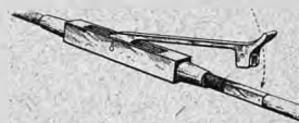
The method provided for adjusting and locking the brake rod of the 20-30 h.p. six-cylinder Hotchkiss.
