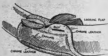
AT OLYMPIA. The new security gaiter shown by Riches and Co. The sketch illustrates the method by which the gaiter may be attached to an air tube inside the outer cover at a weak spot.
