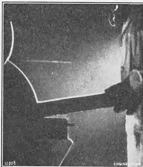
FIG. 2. DUST-FREE ATMOSPHERE WITH MODIFIED COWLING.
