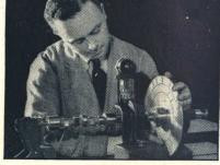
AUSTIN PISTONS are machined oval for positive abrication, and are carefully balanced by pairs for correct weight; on this careful process of selection the smoothness of Austins largely depends.
