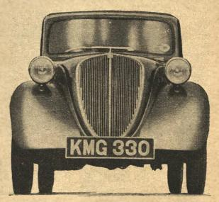
The Fiat has a ground clearance of 61 ins. Access to the power-unit is gained by removing the front cowling—a simple operation.
