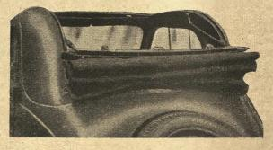
(Above) The head of the Fiat "500" convertible cabriolet rolls right back although the side pillars remain rigid.
