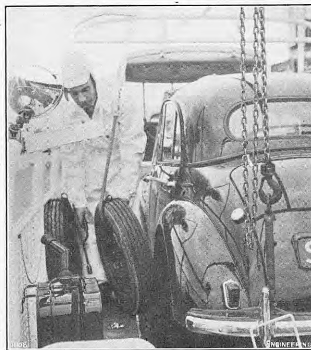
FIG. 2. CHANGING NEAR-SIDE REAR WHEEL ON THE MOVE.
