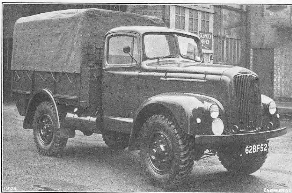
FIG. 14. 1½-TON FOUR-WHEEL-DRIVE LORRY; MORRIS COMMERCIAL CARS, LTD.
