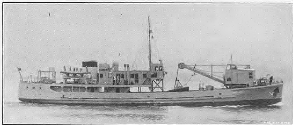
FIG. 6. GRAB-BUCKET HOPPER DREDGE "MERSEY NO. 14."
