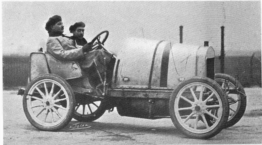
16 h.p. racing Laurin-Klement car which made such a remarkable performance on December 2nd. The bore is 86 mm. and the stroke is said to be about 150 mm.
