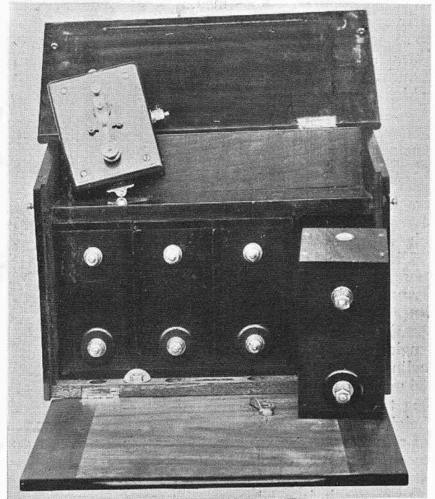
Fig. 2.—The Brooks coil with the trembler block detached and one of the coils withdrawn.
