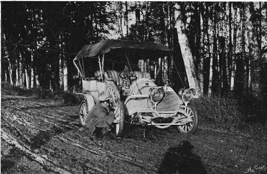
A 16 h.p. Humber changing a wheel (a Humber detachable) in the middle of a forest in Russia. The road is a fair sample of Russian country roads.
