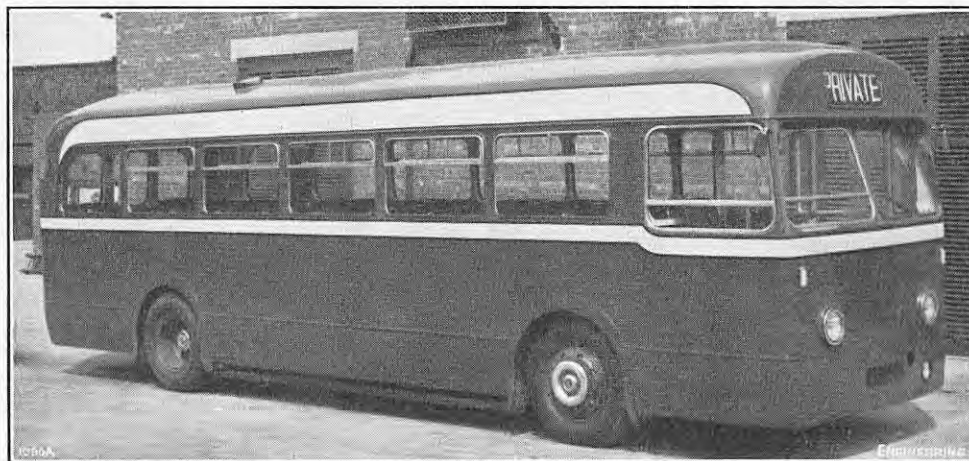
FIG. 1. "TIGER CUB" WITH 44-SEAT BODY BY METROPOLITAN-CAMMELL-WEYMAN MOTOR BODIES, LIMITED; LEYLAND MOTORS, LIMITED.
