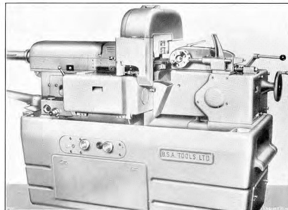
FIG. 83. B.S.A. SINGLE-SPINDLE AUTOMATIC SCREW MACHINE; BURTON, GRIFFITHS AND CO., LTD.
