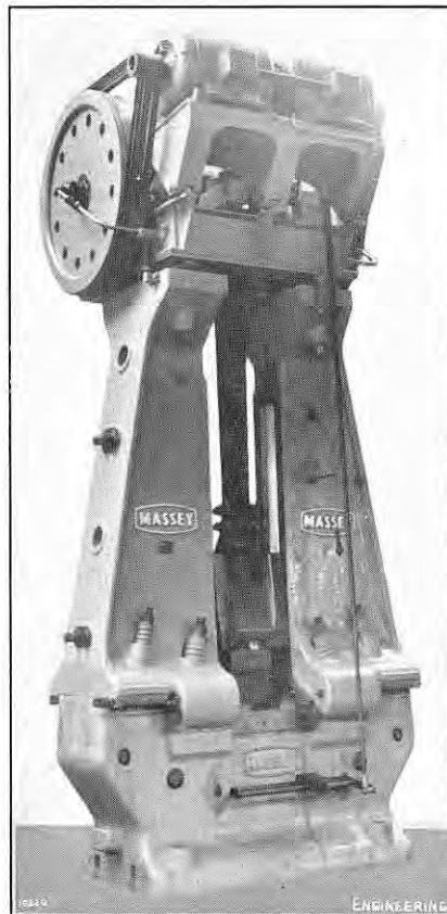
FIG. 77. FRICTION DROP HAMMER; B. AND S. MASSEY, LTD.
