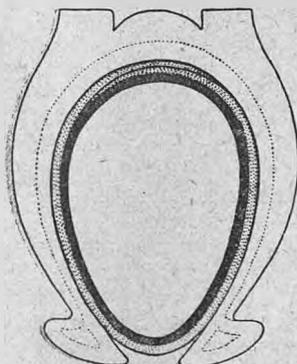
tyre covers may be prolonged to destruction. The liner, for that is the best term by which it can be described, is the outcome of prolonged experiments, and is regarded by the proprietary company as a great factor in the reinforcement of pneumatic tyres. Its construction and application are very clearly exemplified by the accompanying diagram. It is a wrapped tube formed of rubber and fabric, with all
