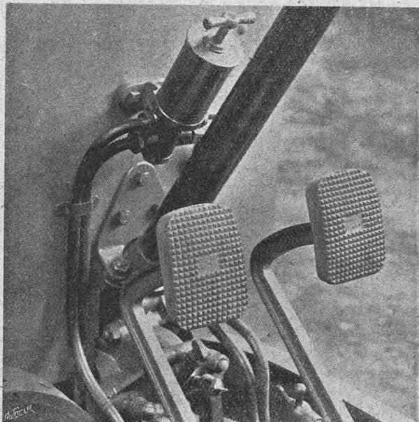
*The United Motor Industries are the British agents for a new rubber pedal cover. These covers are made of Para rubber, and are stocked in numerous shapes and sizes to suit various cars. They are easily fitted, and are designed to obviate the disadvantages of a smoothly-worn pedal, and are most comfortable.*
