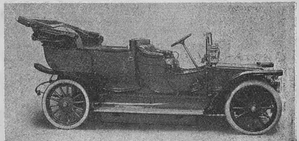
Fig. 3.—The roof-piece, which is made of waterproof cloth material, is mounted on a spring roller in a case on the front of the rear hood. When folded back this extension front becomes invisible. The car thus becomes at will a fully protected or entirely open one.
