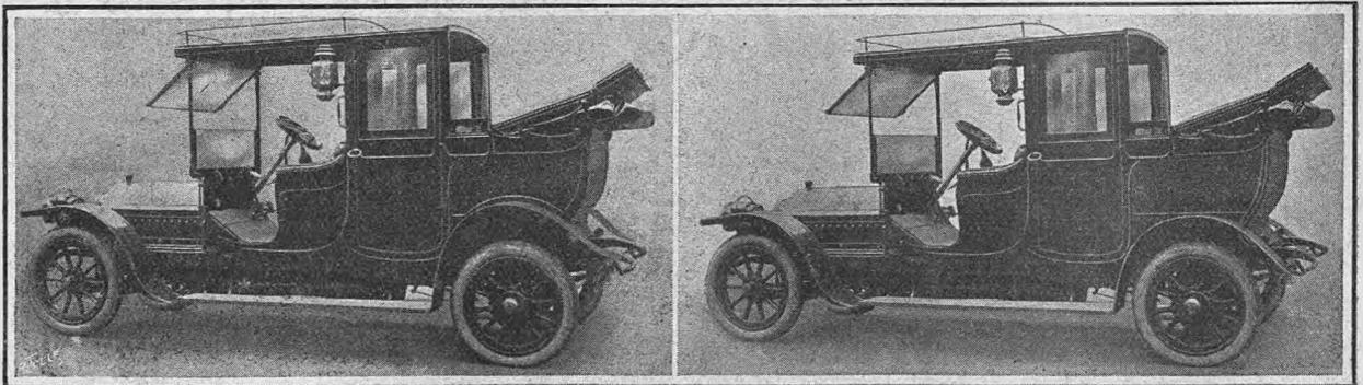
**BODY DESIGN AND CONSTRUCTION.** A 16-20 h.p. Peugeot chassis fitted with Million Quiet body to the order of Mr. James Murray, M.P. The body has a "Victoria" front seat and curved corner pillars at the back. We think the lines of this body would have been improved by the fitting of the rear wings nearer to the wheel and the suppression of the needless curved "paddle box" moulding above the wing. We have altered the print of the right-hand illustration to indicate our idea.
