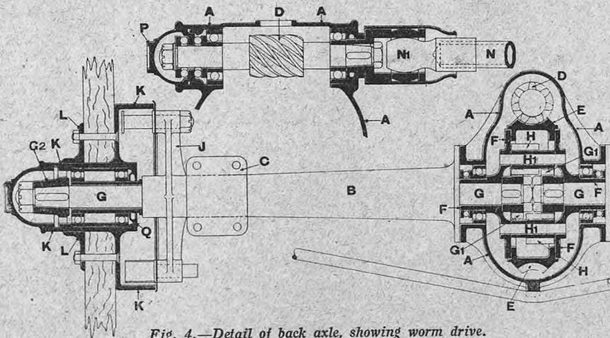
Fig. 4.—Detail of back axle, showing worm drive.
