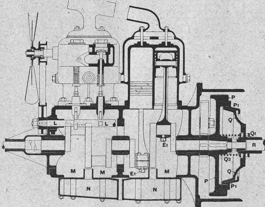
Fig. 2.—Vertical section of engine and crank chamber.
