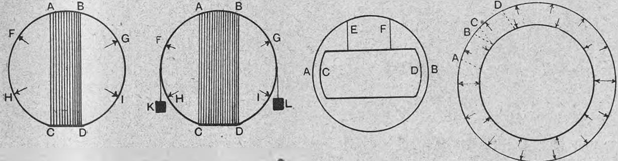
downwards—why should it therefore come downwards? It is forced downwards by its own weight and the load it carries, until this force is balanced by the lifting drag it is receiving from above. The tyre vault cannot readily follow the wheel downwards, and only comes down by being dragged down by the wheel fastened to it, which thus receives its support.
