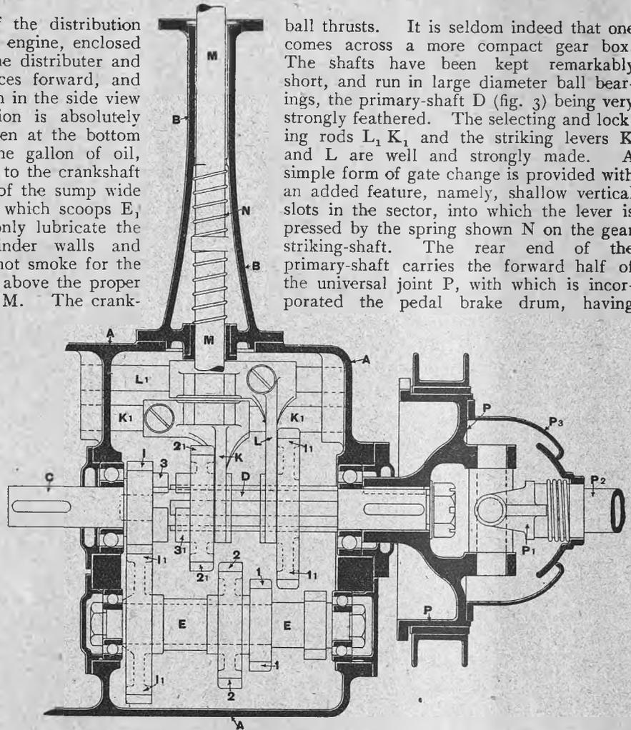
Fig. 3.—Plan of gear box and forward universal joint.
