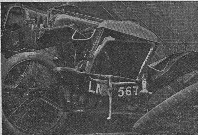
*A front view of the Hon. Ian A. Gordon's car after the cross road accident near Winchester. This gives some idea of the force of the collision and forms a warning to all drivers to cross or enter into a main road slowly. It is interesting to observe that neither of the Rudge-Whitworth front wheels is broken. The back wheels also escaped, though the wooden wheels on the other car were badly damaged, one being completely wrecked, the spokes breaking off like carrots.*
