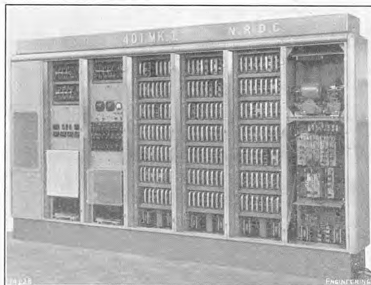
FIG. 9. INTERIOR OF COMPUTER CABINET; ELLIOTT BROTHERS (LONDON), LTD.
