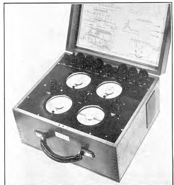
FIG. 16. ALTERNATING-CURRENT TEST SET; SALFORD ELECTRICAL INSTRUMENTS, LTD.
