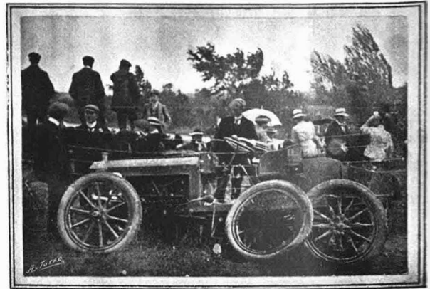
Mr. J. W. Stocks's racer after the accident. The rim of the off front wheel is seen lying against the rear wheel.
