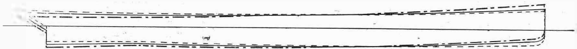
Fig. 1.—Diagram showing the trim with a load of 3 tons in different positions. Total displacement 33 tons. A short table giving the results of the different displacements is given with the article.
