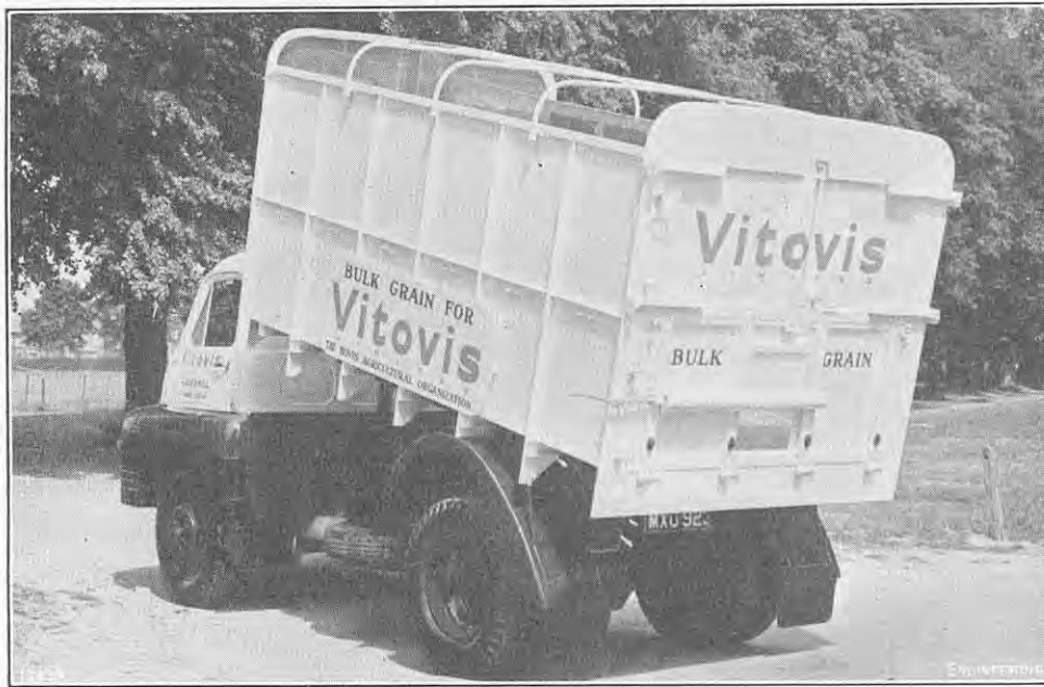
FIG. 1. TIPPING LORRY FOR BULK GRAIN.
