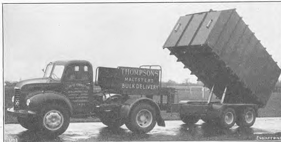
FIG. 2. MALT LORRY WITH CLOSED HOPPER BODY.
