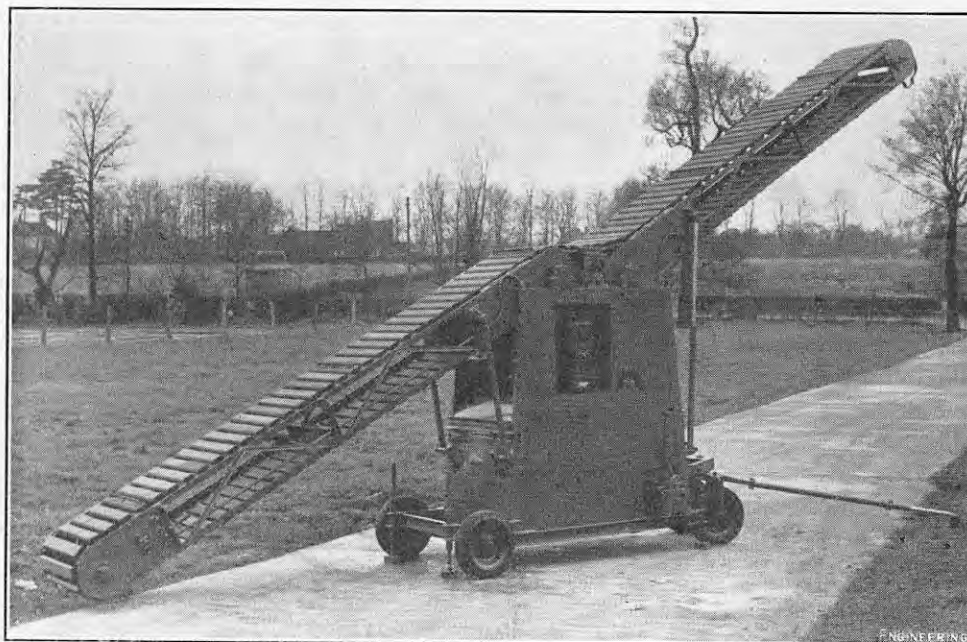
FIG. 22. TRANSPORTABLE CONVEYOR; FOURWAYS (ENGINEERS), LIMITED.
