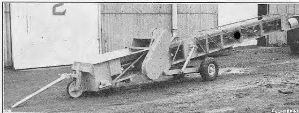
FIG. 21. LIGHT MOBILE STACKER; CRONE AND TAYLOR, LIMITED.
