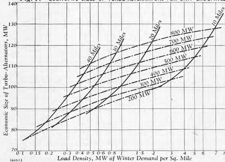
Fig. 7. ECONOMIC SIZES OF TURBO-ALTERNATORS FOR UNIT GROUPING.
