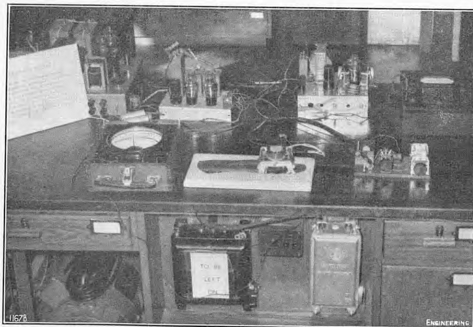
FIG. 3. THICKNESS GAUGE FOR NON-FERROUS METALS.
