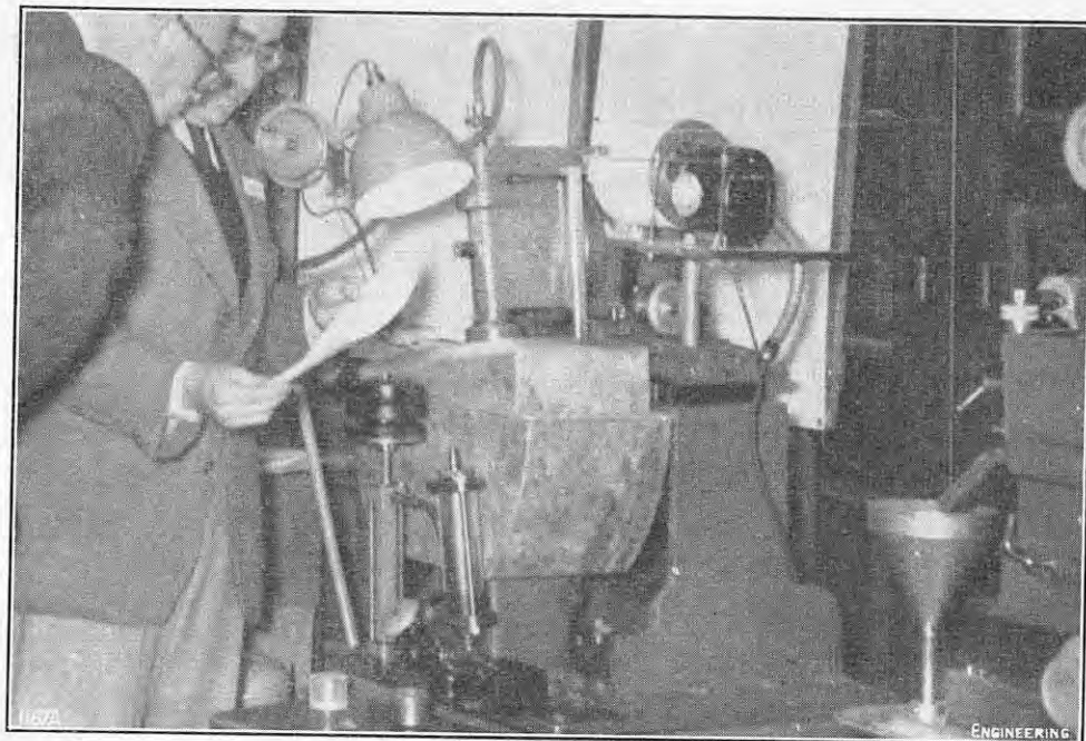
FIG. 1. TEST RIG FOR INVESTIGATION OF GLASS GRINDING.
