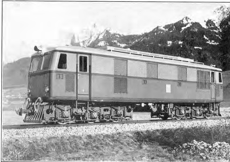
FIG. 11. 960-H.P. DIESEL-ELECTRIC LOCOMOTIVE; THAI STATE RAILWAYS.
