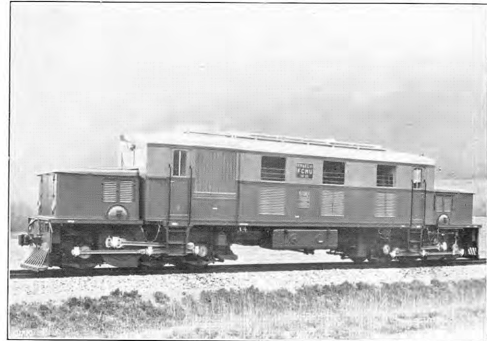
FIG. 10. 730-H.P. DIESEL-ELECTRIC LOCOMOTIVE FOR BOLIVIA.
