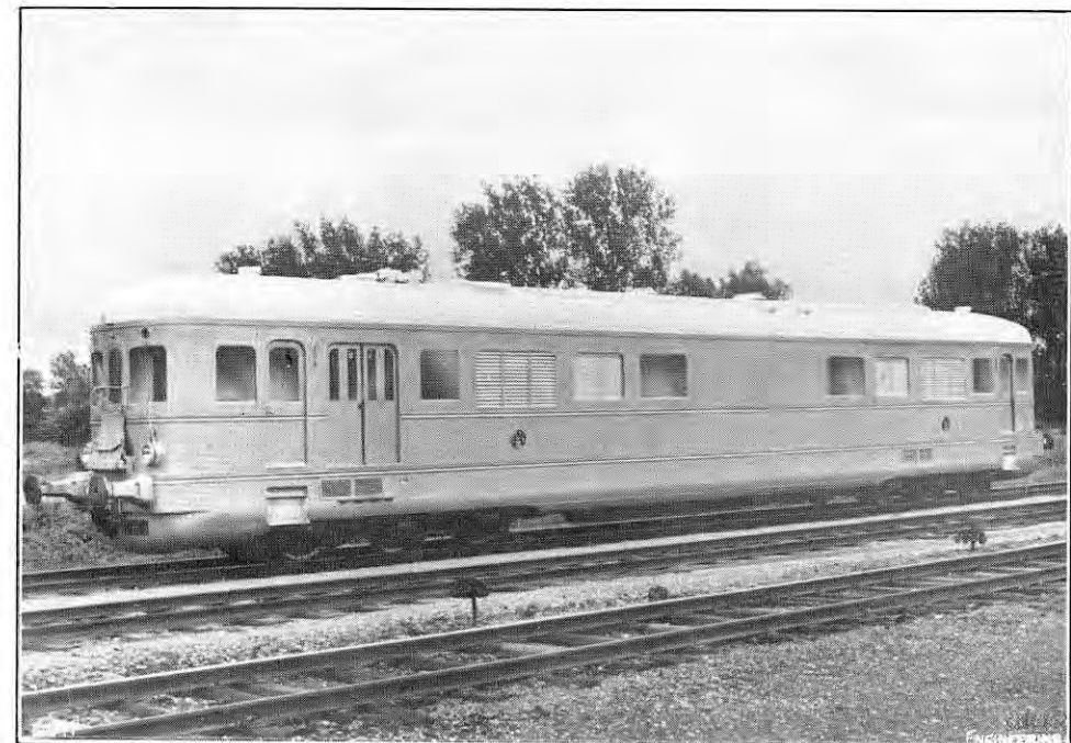
FIG. 12. 1,470-H.P. DIESEL-ELECTRIC LUGGAGE RAILCAR; CHEMINS DE FER ALGÉRIENS.
