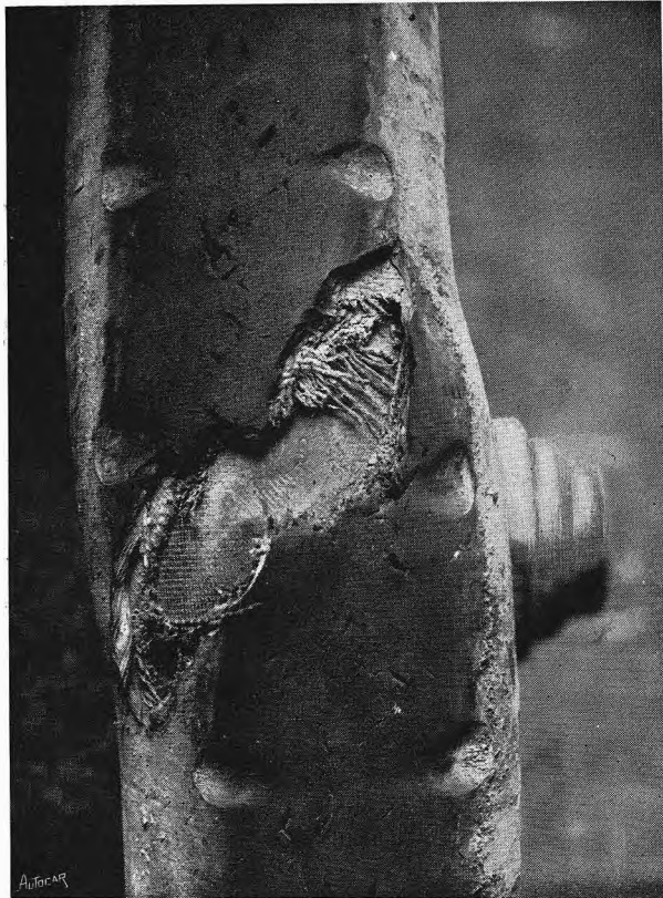
The rent in the cover, exposing the Atlas puncture proof inner case.
