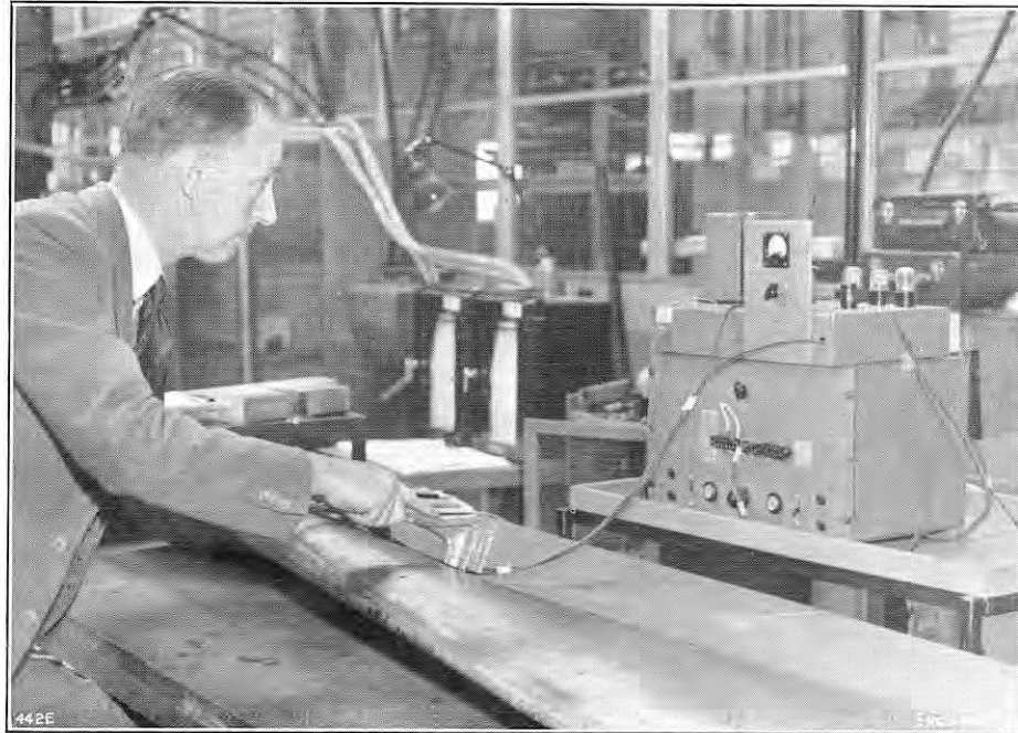
FIG. 17. PROBE-TESTING THE BRAZED JOINT.
