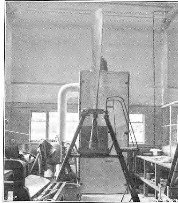
FIG. 18. SWING RIG FOR LACQUERING BLADE INTERIOR.
