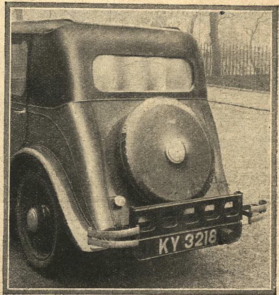
Sweeping lines characterize the rear; luggage can be carried either on the grid or in a large locker inside the tail.
