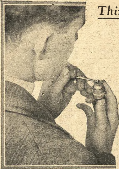
Although slight variations in plug gaps may have little effect, it pays to set the points with a feeler gauge.
