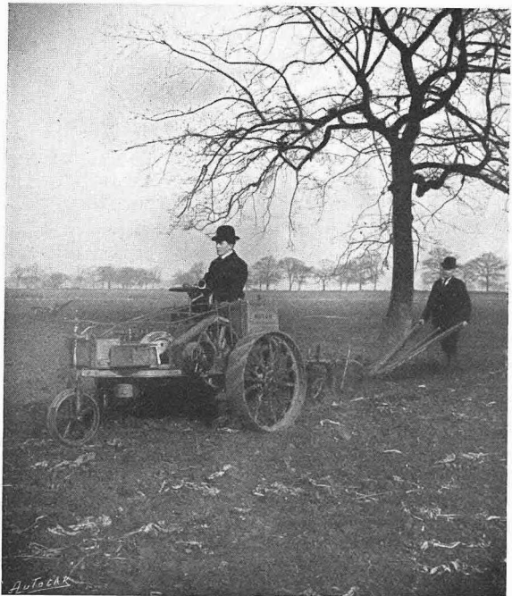
The level agricultural motor drawing a plough. This is only one of the many uses to which it may be put, as it is capable of taking the place of horses in the field for such work as ploughing, mowing, reaping and binding, etc.; in addition to which it acts as a traction for road work, and a stationary engine for grinding, chaff-cutting, etc. The motor is a 10 h.p., governed one of the simplest type, and the upkeep we understand is particularly low. The machine has been designed and made to stand the roughest work.
