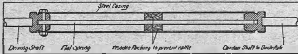
The Marshall-Arter transmission by steel spring. The casing is only held at one end, and thus the give of the spring provides a very flexible drive.
