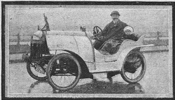
A cyclecar home-constructed by alterations to an old Phoenix quad car.
