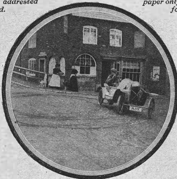
Turning in almost its own length. An illustration of the wide lock on the Sabella tandem cyclecar.
