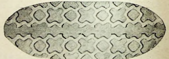
These photographs show the increased area of contact obtained with a low-pressure tyre. The additional adhesion is an advantage.
