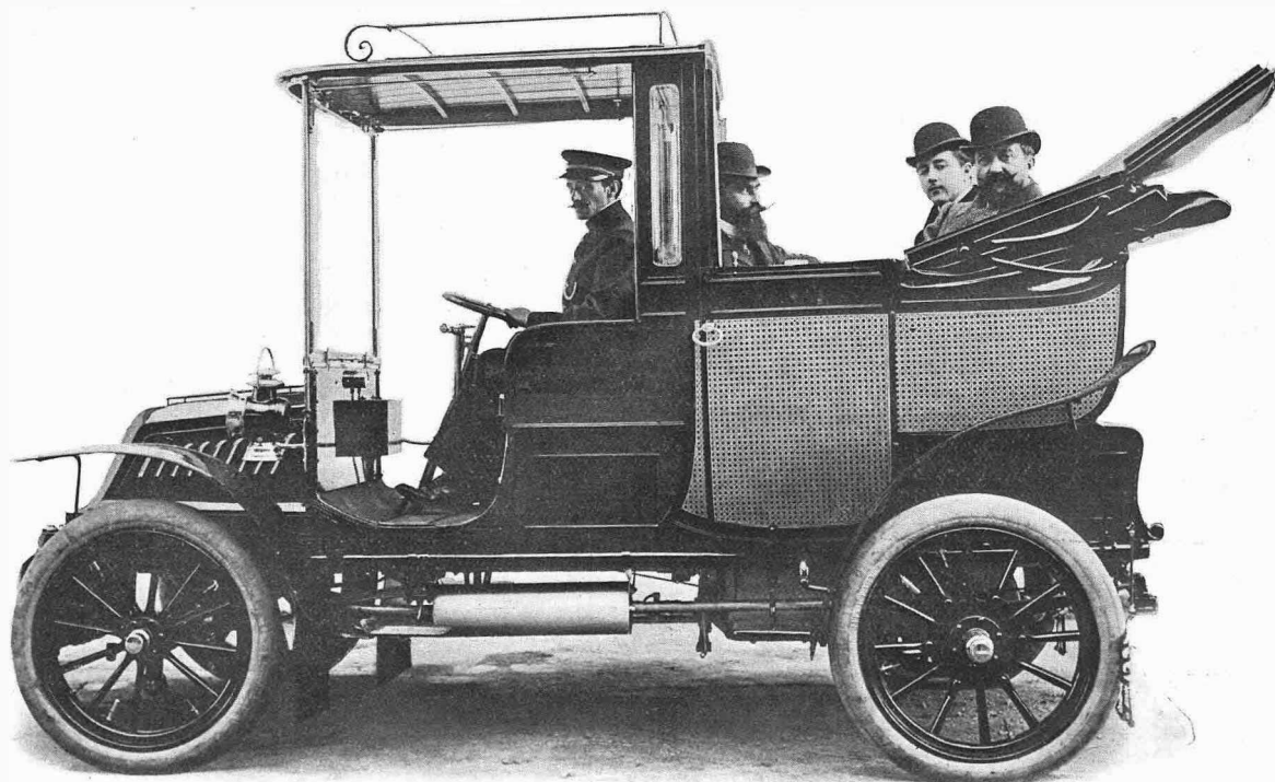
THE 12 H.P. DE DION. This car is a good example of the extended wheelbase type, which is now becoming so general. It permits entrance to the back seats from the side, and with the special front canopy and folding hood which, when up, makes a watertight junction with the back of the canopy, constitutes a most comfortable vehicle which is suitable for use in any weather. This particular landaulette is the property of M. Gailhard, Director of the Paris Opera, who is seated in the back of the car.
