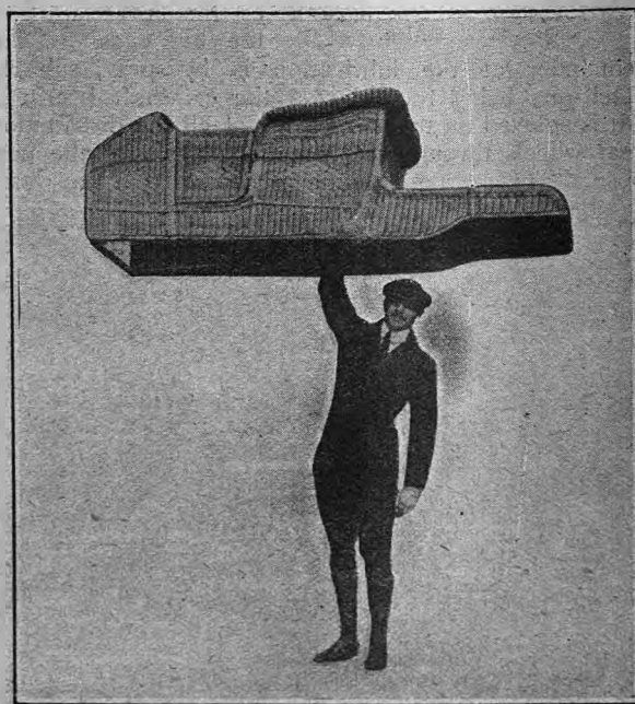
LIGHTNESS IN BODY CONSTRUCTION. A demonstration of the light weight of the basket-work body mounted by the Beacon Engineering Co., Hindhead, Surrey, on their Beacon runabout.
