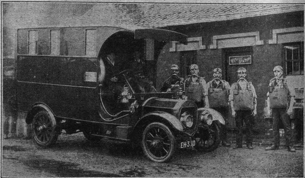
An Enfield van supplied to the North Staffs. Colliery Owners' Association. It has been specially fitted for service at the mining rescue station at Stoke-on-Trent, being arranged for carrying the rescue party and their apparatus.
