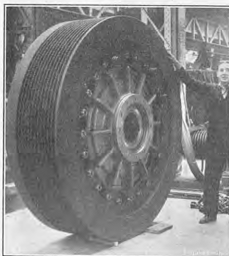
FIG. 8. FLYWHEEL AND CLUTCH ASSEMBLY FOR 1,000-TON HIGH-SPEED PRESS.
