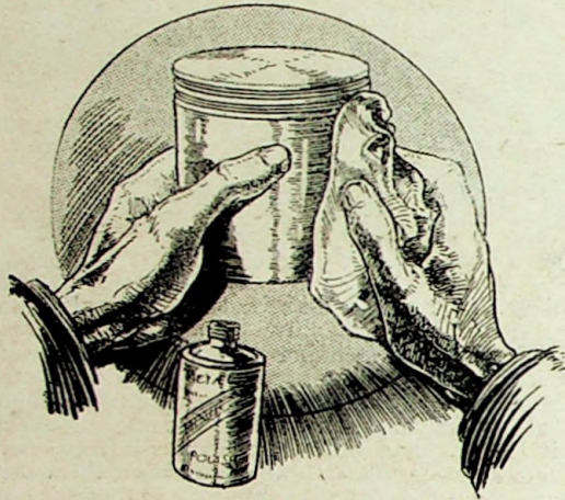
Reducing friction. If the pistons are given a high polish more efficient lubrication is secured.
