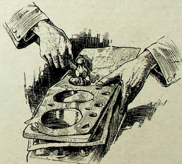
Simple, but efficacious. The only certain method of cutting a perfect washer. The brown paper should be kept well down on the casting.
