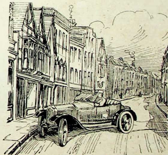
The true cyclecar must have a small turning radius. Many light cars are deficient in this respect.
