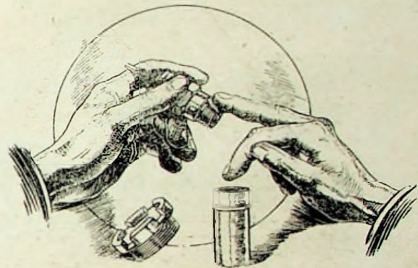
Prevention better than cure. A little graphite applied to the threads of sparking plugs and valve caps prevents them becoming immovable in the cylinder head.
