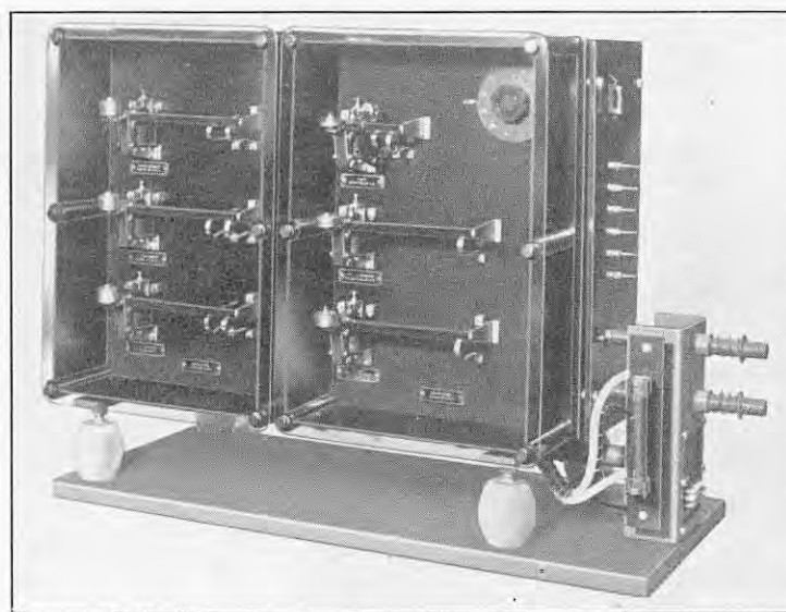
FIG. 7. ELECTRONIC ARC-SUPPRESSION EQUIPMENT.
