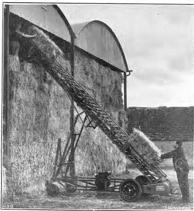
FIG. 13. UNIVERSAL 18-FT. ELEVATOR; A. B. BLANCH AND COMPANY, LIMITED.
