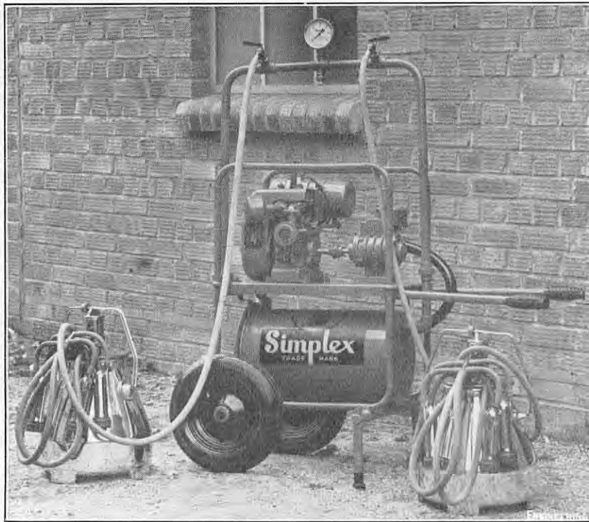
FIG. 7. "UNIVERSAL" PORTABLE MILKING MACHINE; SIMPLEX DAIRY EQUIPMENT COMPANY, LIMITED.
