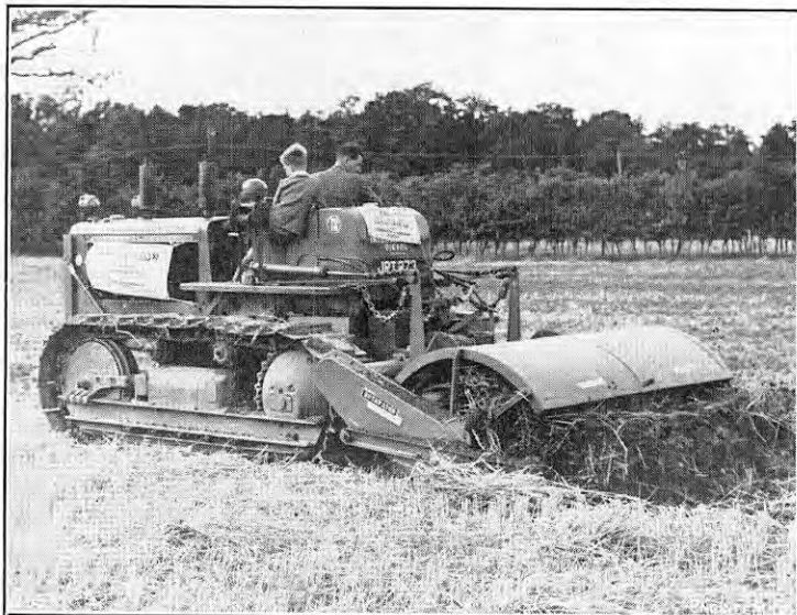
FIG. 11. INTERNATIONAL TRACTOR FITTED WITH ROTARY HOE; ROTARY HOES, LIMITED.
