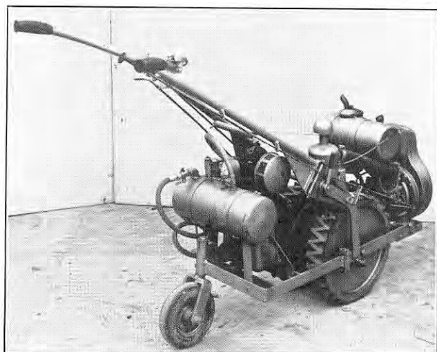
FIG. 15. "BANTAM" ROTARY HOE FITTED WITH HYMATIC COMPRESSOR; ROTARY HOES, LIMITED.
