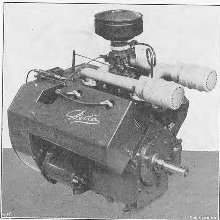
FIG. 1. 19-H.P. FOUR-CYLINDER V-TYPE PETROL ENGINE.
