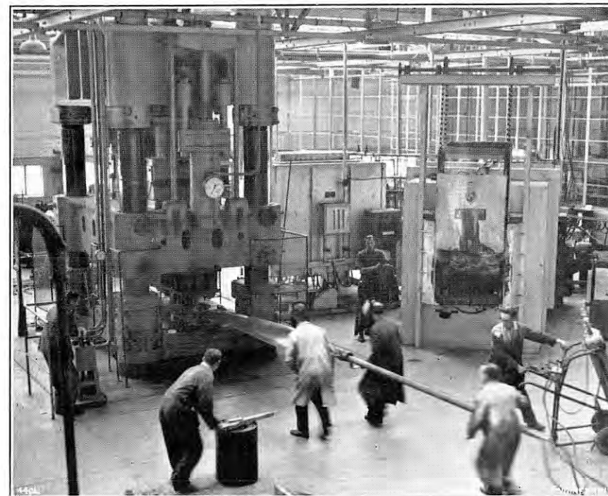
FIG. 11. TRANSFERRING BLADE SHELL FROM FURNACE TO PRESS.
