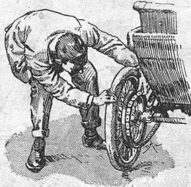
How to remove the belt (from the rear pulley).
