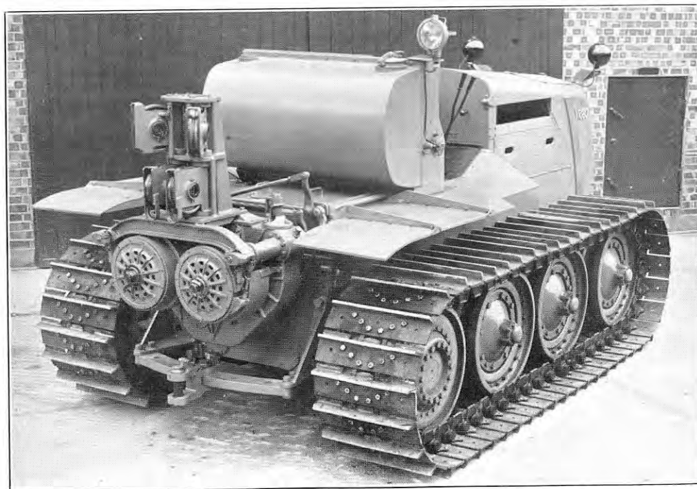
FIG. 4. CABLE CONTROL UNIT ON TRACTOR; JACK OLDING AND COMPANY, LIMITED.
