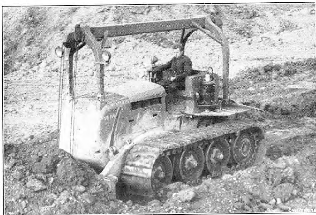
FIG. 3. VICKERS TRACTOR WITH CABLE-CONTROLLED DOZER; JACK OLDING AND COMPANY, LIMITED.
