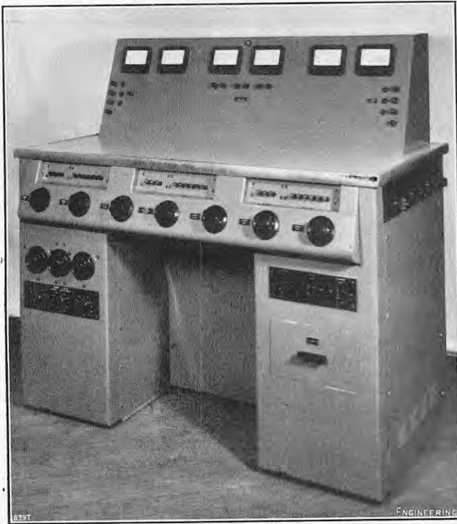
FIG. 14. POLYPHASE METER-TESTING SET; FERRANTI, LTD.
