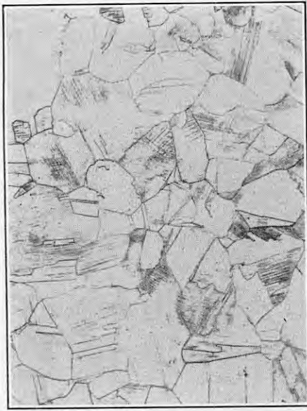
FIG. 1. SINGLE-PHASE ALUMINIUM BRONZE. \times 100 .
