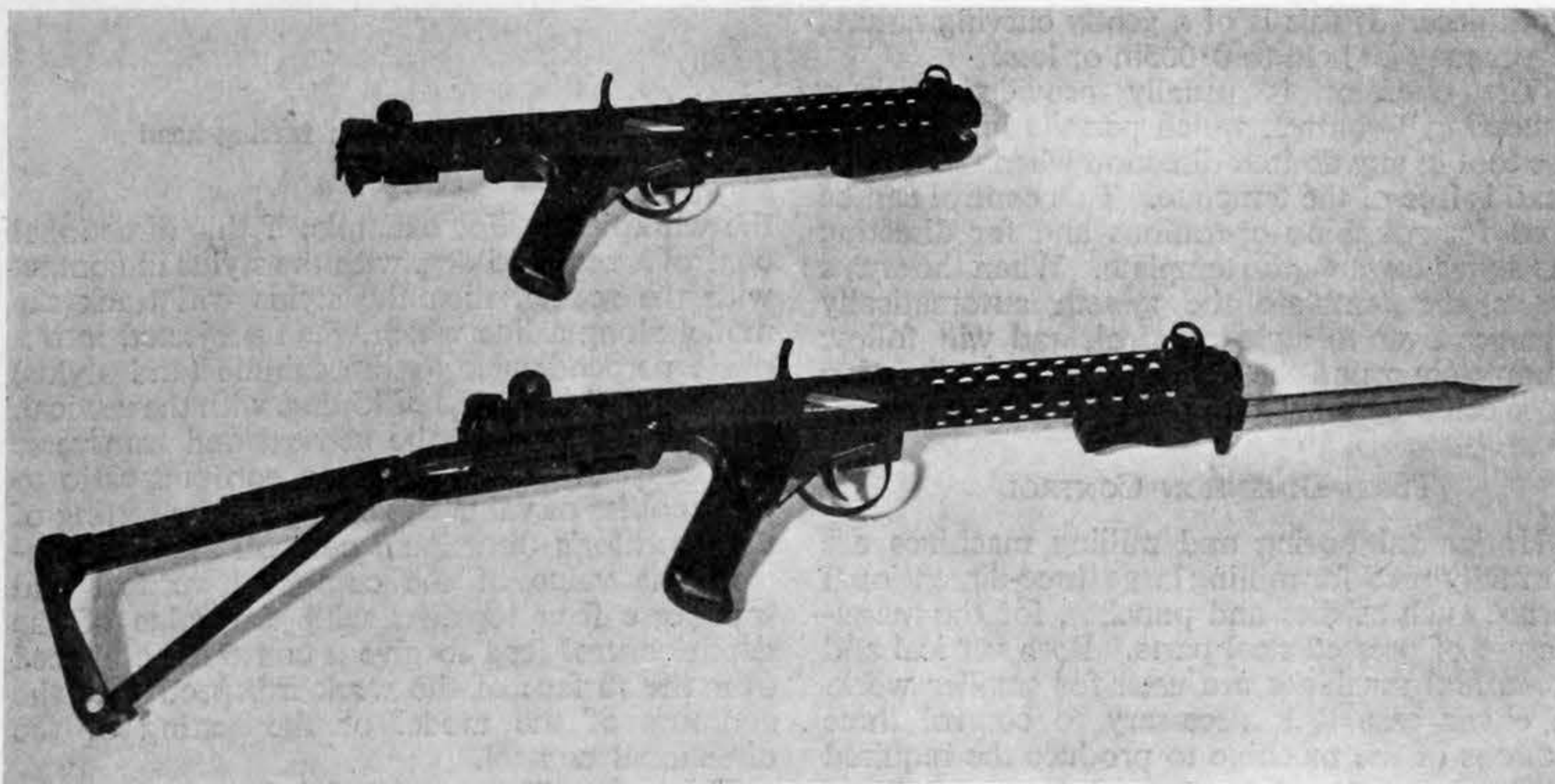
Fig. 1—The Sterling sub-machine gun shown with butt folded and with butt fully extended with bayonet attachment
