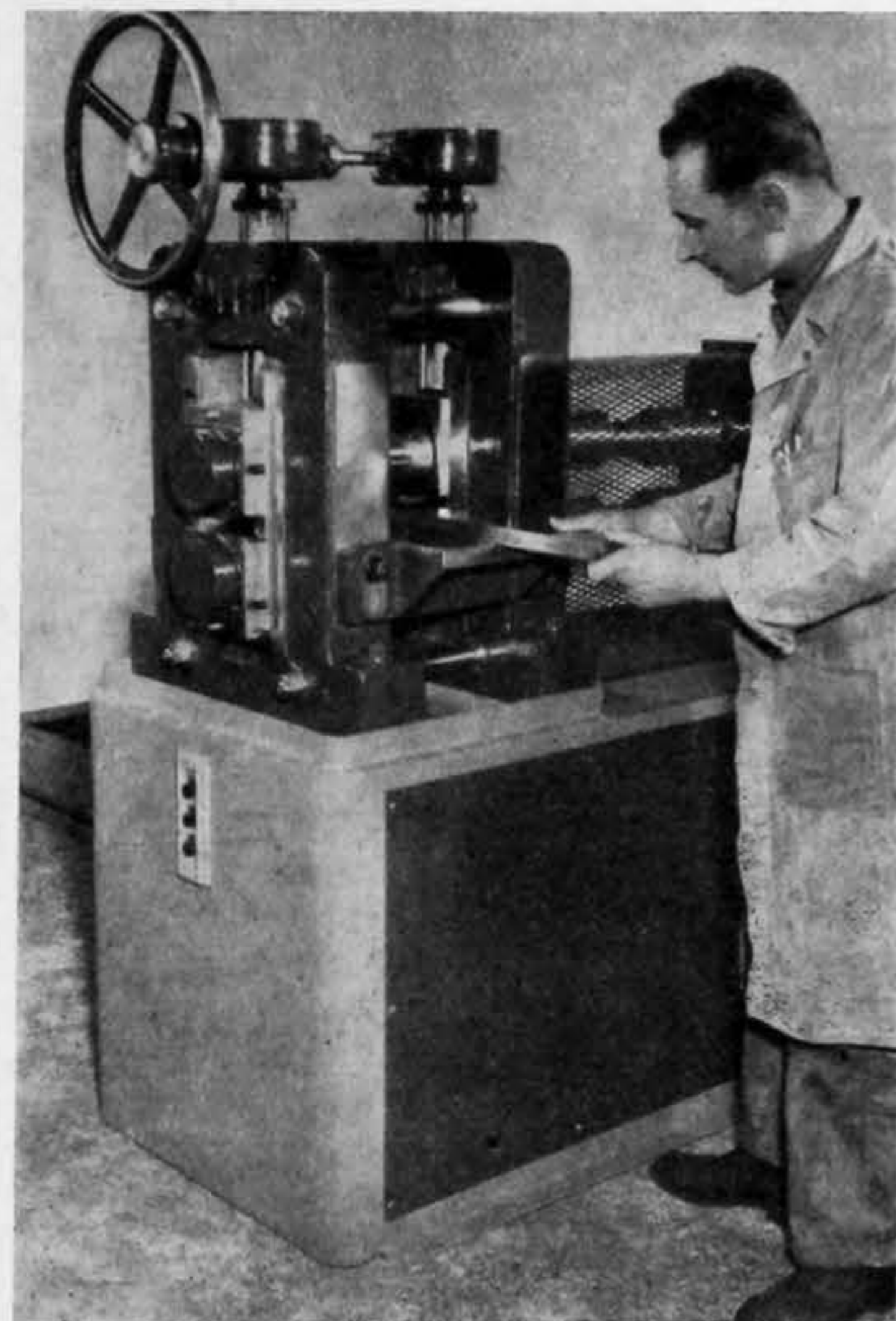
Fig. 3—Ingot break-down on two-high/four-high combination rolling mill, using the two-high arrangement
