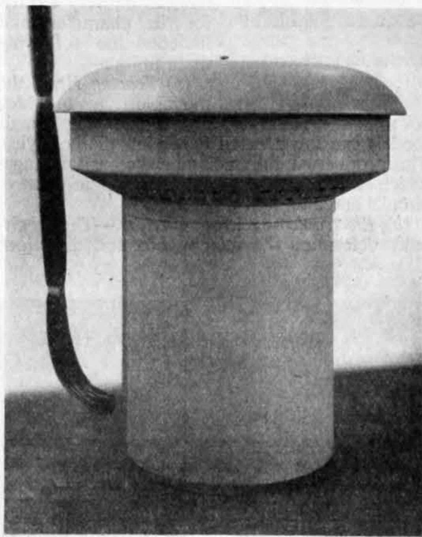
Fig. 9—Thermostatically-controlled drum container for the longer mercury delay lines. This container is positioned at any convenient distance from the main cubicle assembly and control desk
