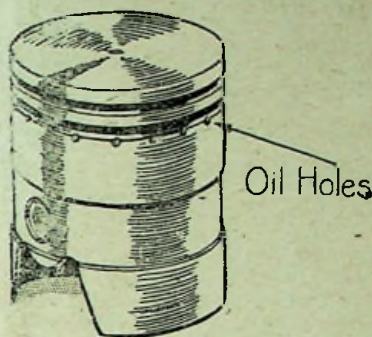
The racing-type piston showing the upper and the lower grooves.
