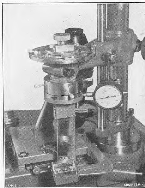
FIG. 10. BLADE-HOLDING FIXTURE AND SUPPORTING COLUMN.
