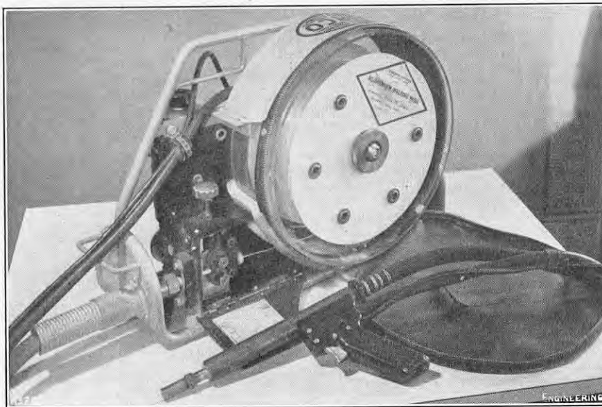
FIG. 2. REGULATOR FOR ELECTRODE WIRE AND WELDING GUN.
