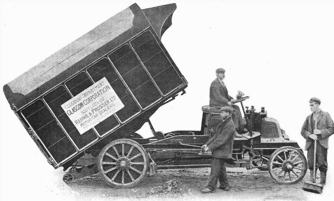
One of the new Glasgow tip waggons. The vehicle is built by Messrs. Milnes-Daimler, Ltd., and with the exception of the body work and the apparatus for tipping the load it is the same as the ordinary 2½ ton Milnes lorry. The two-cylinder engine has a bore of 105 mm. and a stroke of 130 mm. Three tons are frequently carried. Our illustration is made from a photograph taken when the vehicle was undergoing its trials in Glasgow before the cleansing department of the Corporation.
