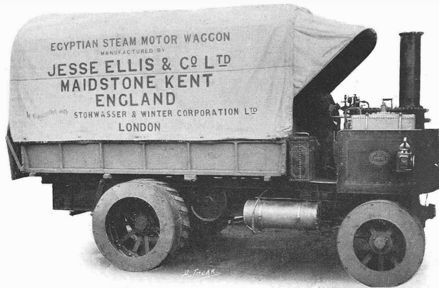
The Jesse Ellis steam wagon, which was recently shipped to Egypt. The special construction of the wheels to make them fit for running over the loose sandy tracks will be noted. In other respects the vehicle is of the standard type turned out by Messrs. J. Ellis & Co., Ltd.
