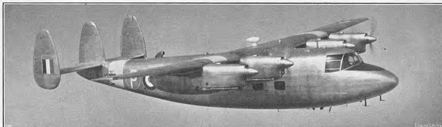
FIG. 12. "MARATHON" NAVIGATION TRAINER AEROPLANE; HANDLEY PAGE, LTD.
