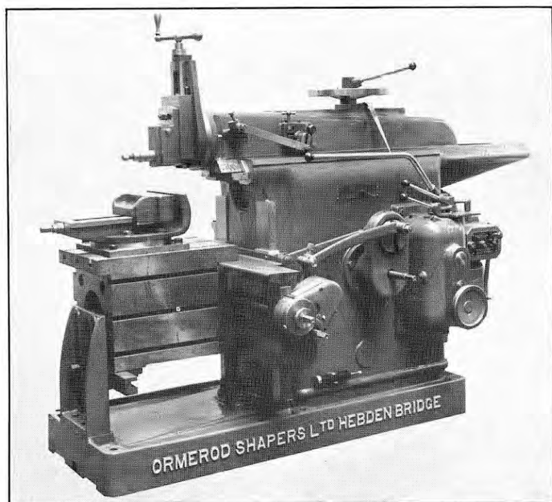
FIG. 110. 12-IN. ORMEROD SHAPER; KITCHEN & WADE, LTD.
