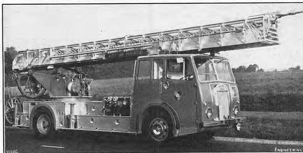
FIG. 11. TURNTABLE FIRE ENGINE; DENNIS BROTHERS, LTD.
