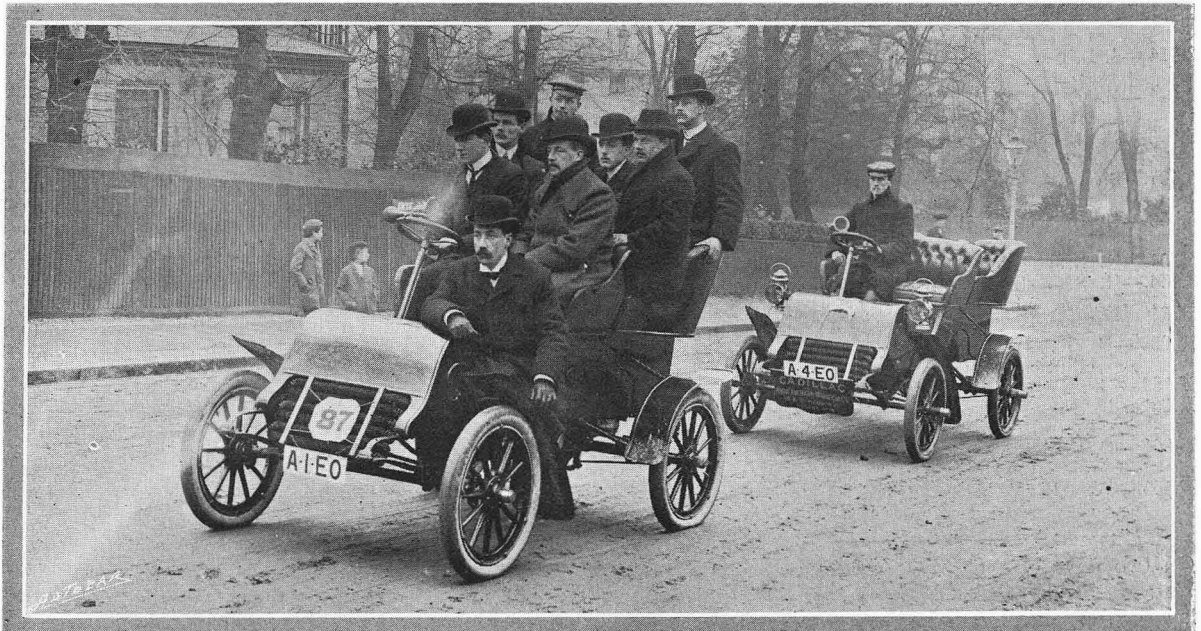
The 6½ h.p. Cadillac climbed the hill known as Crystal Palace Park Road with eight passengers on board—double its proper load. The hill referred to is the long one approached by running down the grounds from the north tower and then turning sharply to the left at the bottom gate. Competitors in the 1,000 miles trials know the hill very well. They descended it on all occasions when they went south or east from the Crystal Palace on their daily runs, as it is the main road from the Palace Parade to Beckenham. It is a fine wide road, and sometimes when three or four cars were making trial runs up it last week it looked as though a hill-climbing competition was in progress. It is whispered that appearances did not belie the fact.
