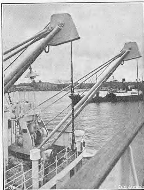
FIG. 2. ELECTRIC CARGO CRANES.
