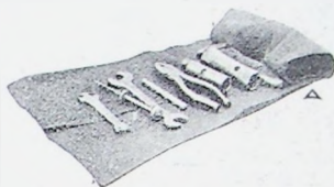
A strip of cloth cut from a discarded pair of trousers makes a very serviceable tool roll.
