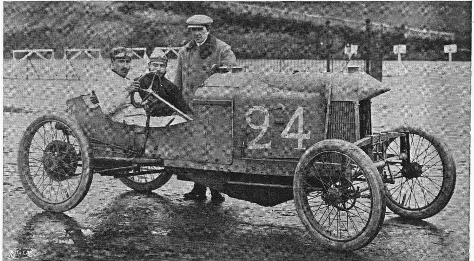
M. Naudin at the wheel of the single-cylinder Sizaire-Naudin car which covered 100 miles on Brooklands Track at an average speed of 65 miles an hour. Standing beside the car is Mr. Charles Jarrott, whose firm have long since taken up the English agency for these speedy little cars.
