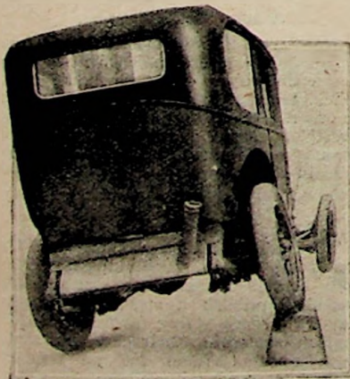
Showing the immunity of a Gordon England three-point suspended body from flexing when the chassis is distorted.
