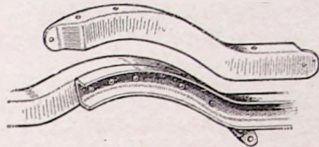
How a curved side member can be lengthened. The joint could be hidden by a sheet-metal cover.
