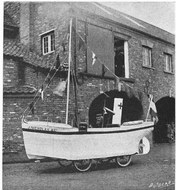
Bridgwater Guy Fawkes carnival is a great event as great if not greater than the celebrated Lewes 5th of November celebration, and one of the most effective items in the Bridgwater procession was Mr. R. J. Sully's 3½ h.p. De Dion, decorated as a steamboat. The propeller was driven by a pulley fastened on the differential gear. The car has carried three average weight people and luggage eighty miles through Devon and Somerset in six hours without a stop. We have to thank Mr. W. H. Glover for the photograph from which our illustration is made.
