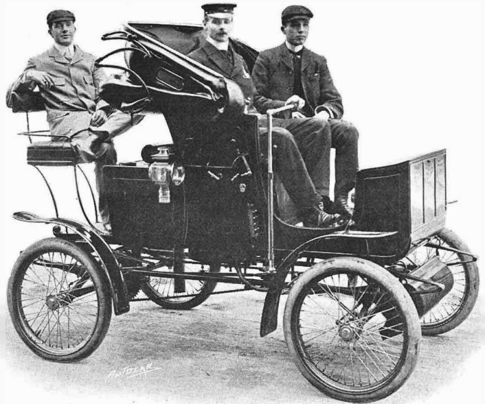
This is a new type of Locomobile, and only a limited number have been made. The vehicle runs with extreme smoothness, almost as though it was hung on C springs, and has a petrol capacity of sixty to eighty miles, and carries sufficient water for a thirty miles run. It has been bought by Mr. Russell Skinner, who is shown at the helm.
